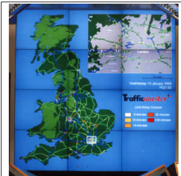
Figure 3: The Trafficmaster control centre collects all the Sensor network and manually Entered Data to construct an integrated picture of the traffic flow for the whole of the UK.
