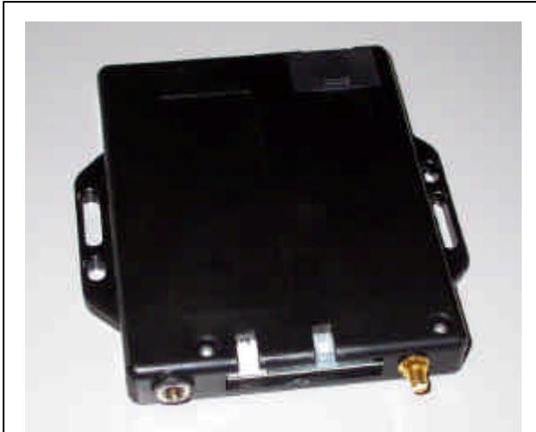
Figure 2: In-vehicle products for vehicle probe data may be hidden "black-box" units or integrated with other driver information systems (Smartnav satellite navigation unit shown above).
